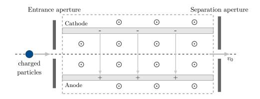
Figure 1: Wien filter's functional principle
