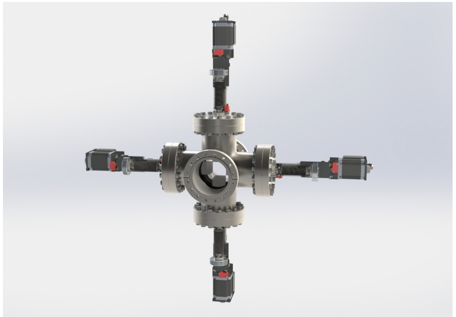
4-Jaw slit system, each slit can be moved individually.
