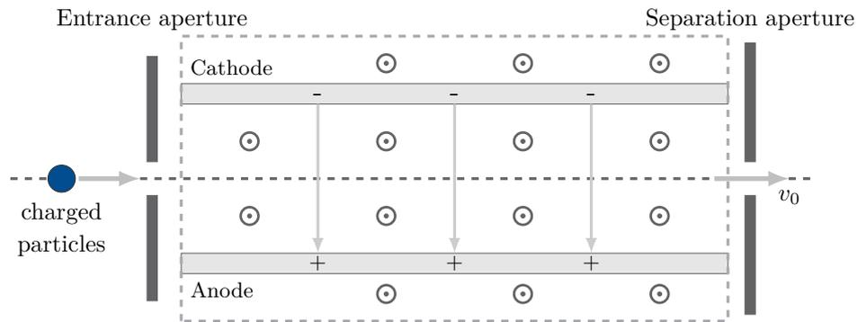
Figure 1: Wien filter's functional principle
